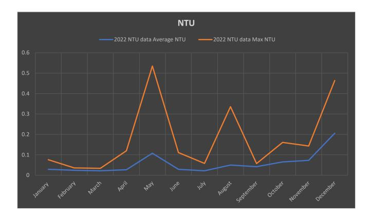
Due to the remote nature of the environment and the quality of the water from our springs, we have consistently low turbidity levels. Occasional high readings are observed, which typically coincide with heavy rain events, storms or rapid spring melts. As shown in the graph above, average values are generally well below 1.00 NTU.
