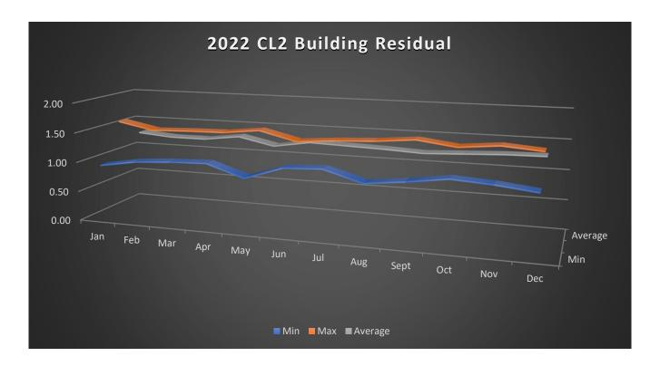
As chlorinated water travels through the distribution system, the chlorine available for disinfection will decrease. It is either used up by any organics or contaminants found in the distribution system, or it dissipates if water sits around for too long. It is important that potable water maintains a measurable chlorine residual throughout the entire system.
